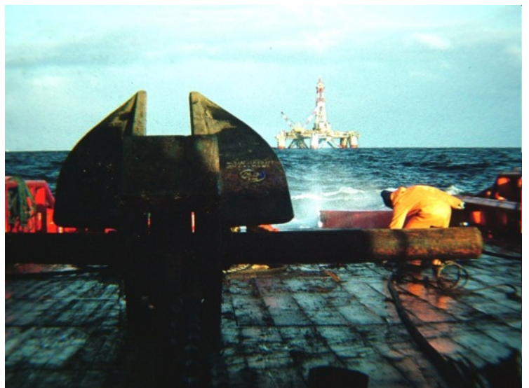
A Rig anchor on the deck of an anchor handling vessel.
